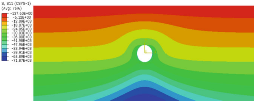
Fig. 6 Contour of tangential stresses in low plastic soil (ML)
