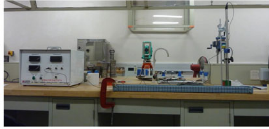
(a) Photo of the imperfection measurement setup
