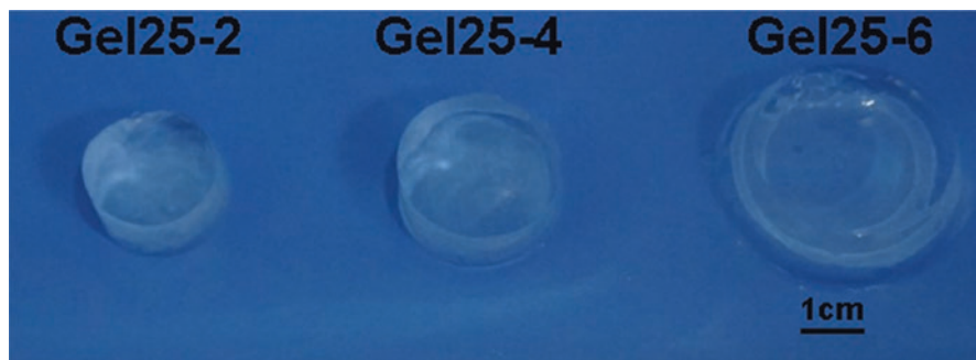
Fig. 10.12 Photographs of QC/cellulose hydrogels after swelling equilibrium in distilled water. (Source: Na et al. (2017) copyright © 2017 with permission from Elsevier B.V.)
