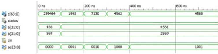
Fig. 7 Arithmetic operations of 32-bit hybrid ALU
