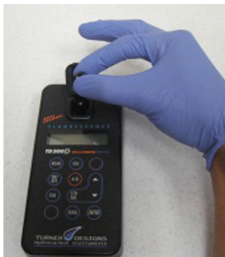
Fig. 2. TD-500D Oil-in-Water analyzer
