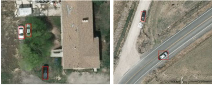
Fig. 4 Examples of small size vehicles detected in VEDAI images by the proposed architecture. The detected vehicles are bounded by red boxes
