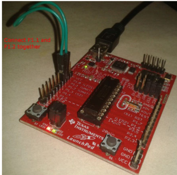
Fig. 6 Loop-back mode in MSP430G2553
