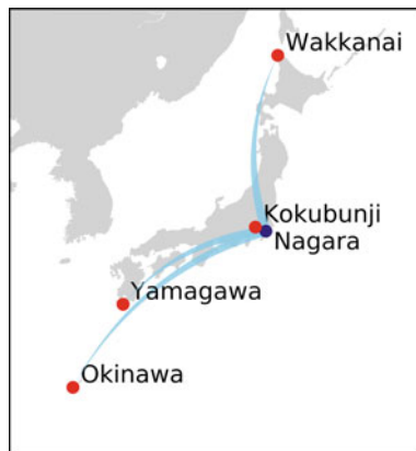
Fig. 7. Location of Tx (dark blue circle), planned Rx stations for the campaign (red circle), and NICT ionosonde stations (red circle). The light blue strips show the possible radio path of each radio link
