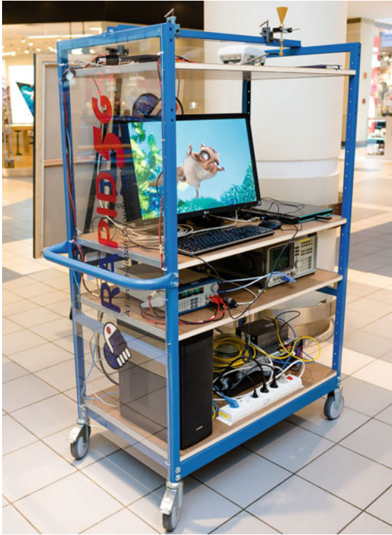
Fig. 11. RAPID5G demo vehicle used as mobile unit in the shopping mall, containing a receiver horn antenna, a RF amplifier, a SBD detector, a baseband amplifier a SDI-to-HDMI scalerbox and a 4 K high resolution screen to display the received video stream
