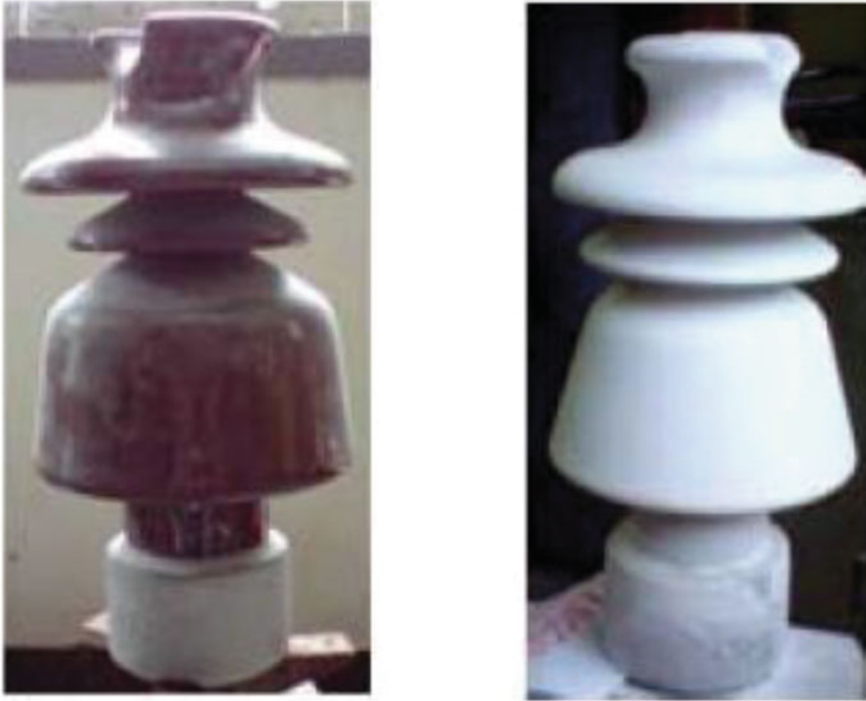
Fig. 5 Pictures of non-coated [left] and RTV-coated [right] samples
