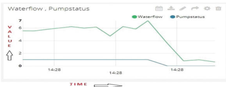
Fig. 3 Graphical representation of uploaded values of flow rate and status of the pump
