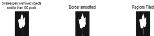
Fig. 5 Morphological operations on the image
