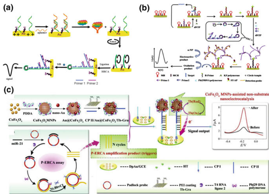
Fig. 7.5 a HRCAs-based electrochemical biosensor for PDGF-BB detection. Reproduced from Wang et al. (2013) by permission of The Royal Society of Chemistry. b Electrochemical DNA biosensor based on the cascade signal amplification of hairpin-mediated CSD and HRCAs. Reprinted from Li et al. (2016). Copyright 2016, with permission from Elsevier. c Schematic illustration of P-ERCA assay and \text{CoFe}_2\text{O}_4 MNPs assisted no substrate nanoelectrocatalysis for miR-21 detection. Reprinted from Yu et al. (2017). Copyright 2017, with permission from Elsevier
