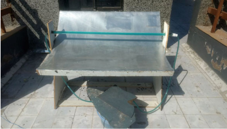
Fig. 1 Setup of parabolic trough collector
