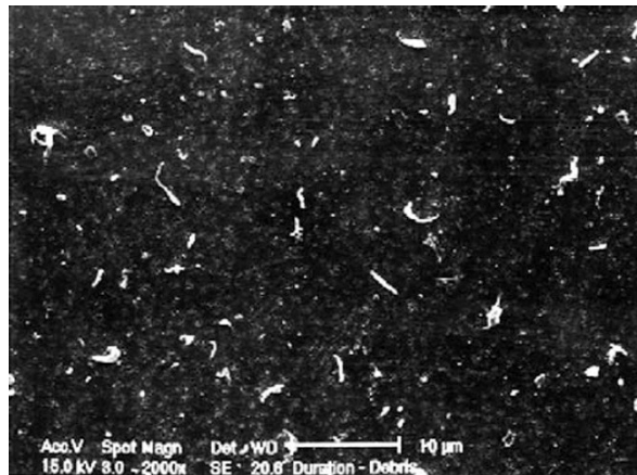
Fig. 8.36 Hip simulator Duration ® UHMWPE acetabular liner wear debris. (Reprinted from Ref. [84], Copyright 2005, with permission from Elsevier)
