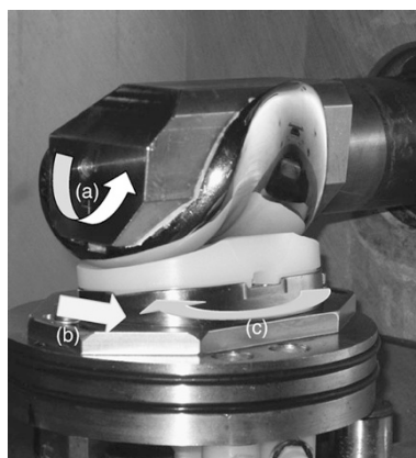
Fig. 2.20 Anatomical positioning of components in the hip simulator. (Reprinted from Ref. [79], Copyright 2005, with permission from Elsevier)
