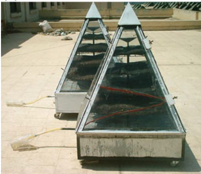
Fig. 13 a Schematic view and b photographic view of solar glass pyramid still [33]
