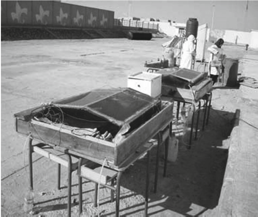
Fig. 5 Two identical single-basin double-slope solar stills [25]
