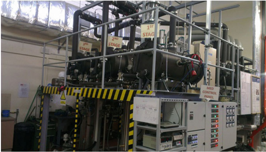
Fig. 31 A three-stages MEDAD experimental unit built in NUS [27, 35]
