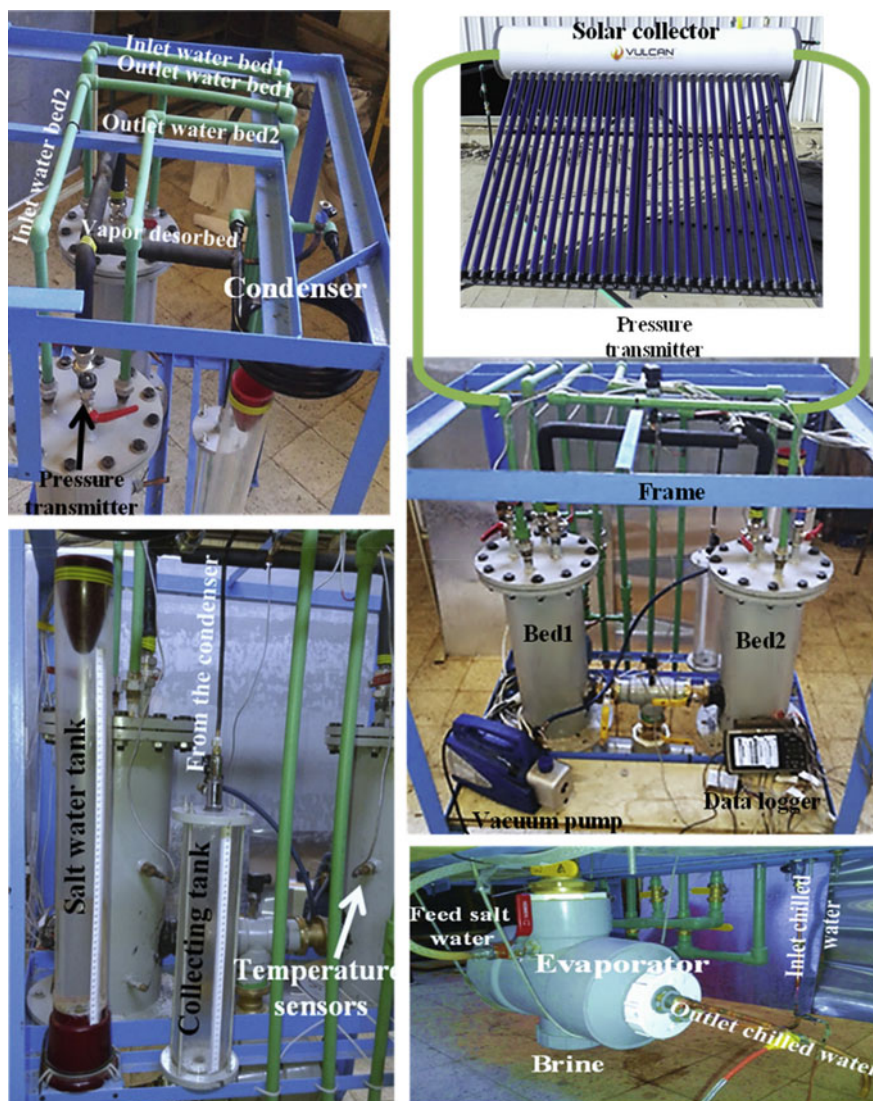
Fig. 26 Photographs of the ADC system built at Sohag University, Egypt [4]
