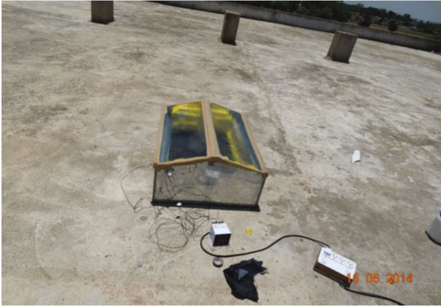
Fig. 28 Solar still with black coated tray [14]
