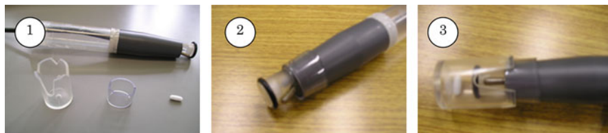
Fig. 4.2 Setup of DO electrode
