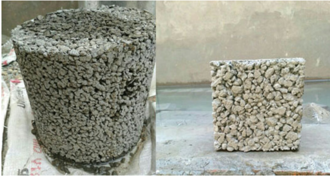
Fig. 1 Pervious concrete cylinder and cube
