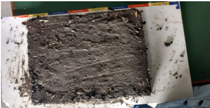
Fig. 1 Wall 2 made of soil and rice husks
