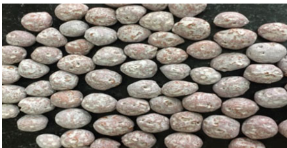
Fig. 1 Actual photograph of freshly coated TiO 2 clay beads
