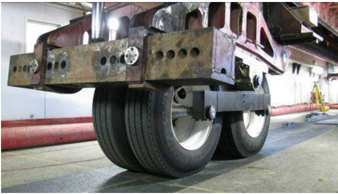
Fig. 5 Tandem-axle dual wheel gear used in ERDC tests
