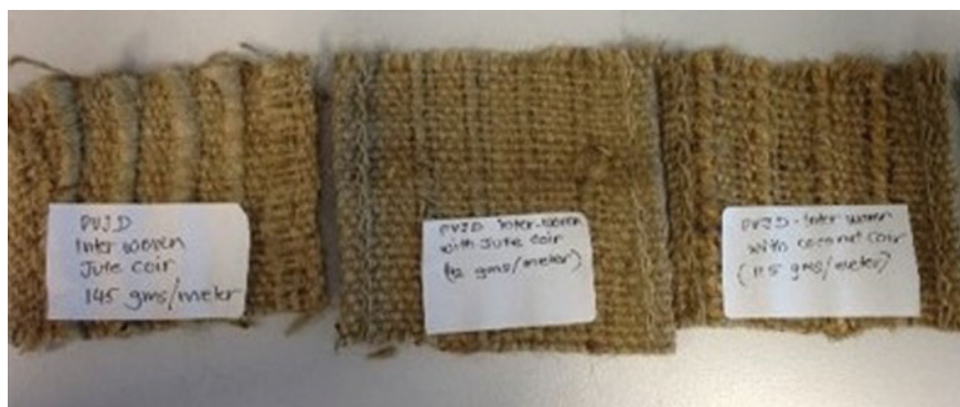
Fig. 1 Jute drains used in the study (drain 1, 2 and 3 from left to right as per Table 1)
