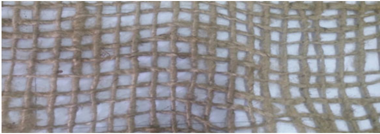
Fig. 2 Open mesh woven jute geotextile
