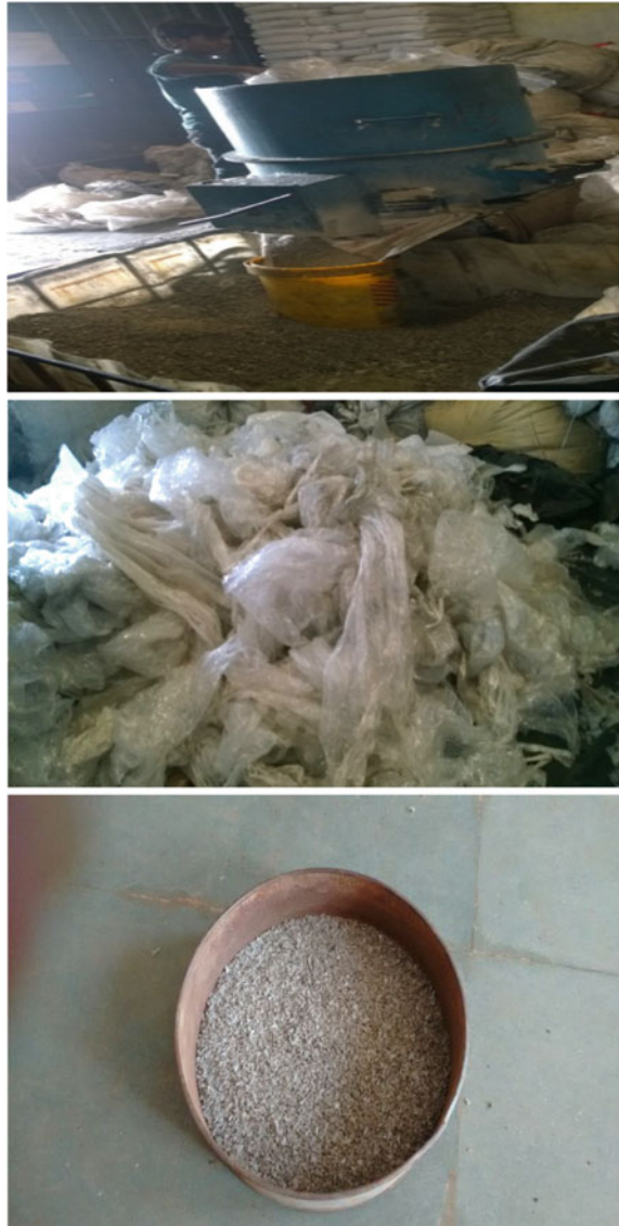
Fig. 1 Plastic shredding machine and shredded plastic
