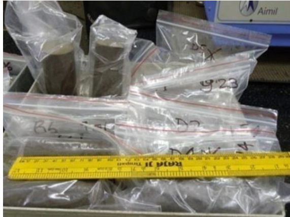
Fig. 4 Storage of samples for curing
