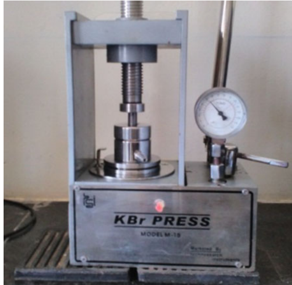
Fig. 2 Pelletizer equipment for sample preparation
