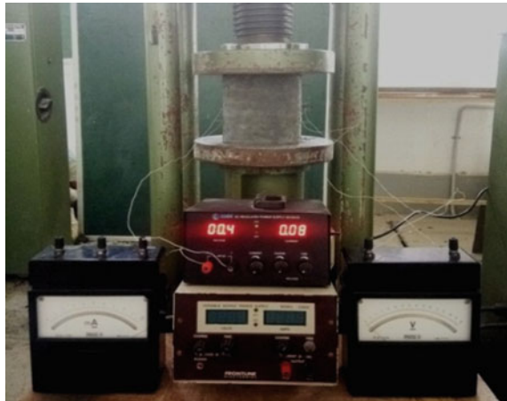
Fig. 4 Uniaxial electrical test arrangement
