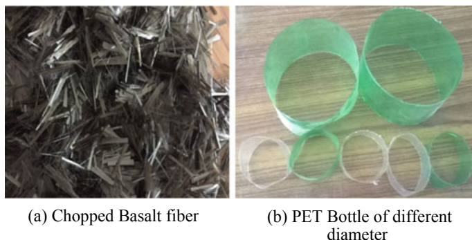
Fig. 1 Fibre PET bottle used in the study
