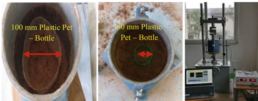
Fig. 3 Plastic confinement preparation and CBR test performed through online DAQ
