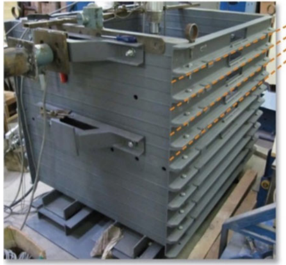
Fig. 8 Multi-level shear box
