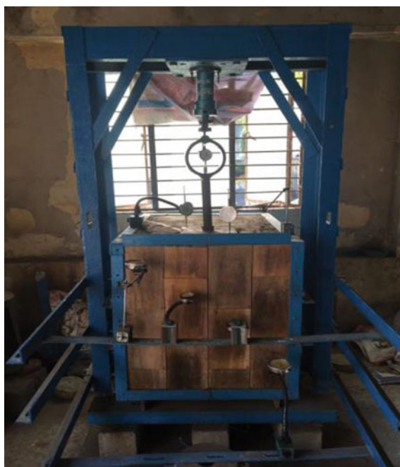
Fig. 4 Reinforced earth wall test model
