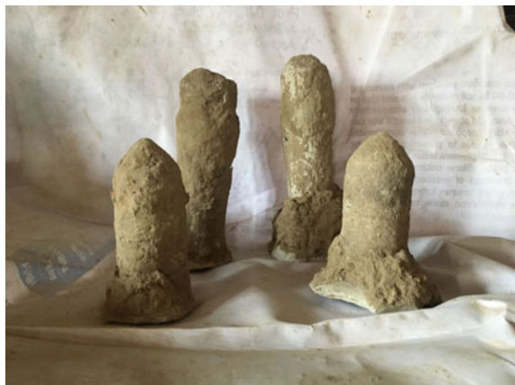
Fig. 4 Extracted soil–cement columns
