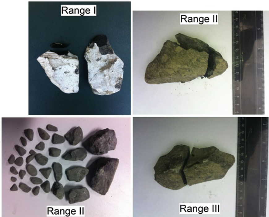
Fig. 9 Typical images of particle breakage (modified after Sun et al. 2016)
