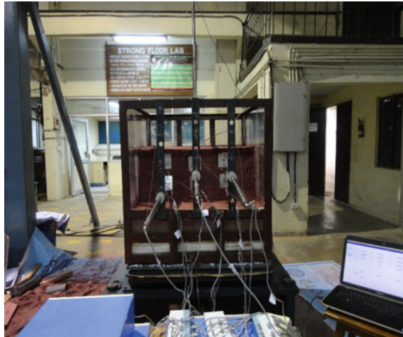
Fig. 1 Front view of complete shaking table test setup
