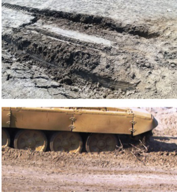
Fig. 15 Heavy tracked vehicle rutting heavily into the soil; above picture shows depth of ruts
