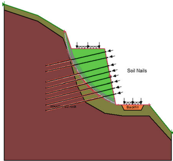
Fig. 3 Prediction of FOS > 1.5 with eight rows of designed length nail (Case-B)
