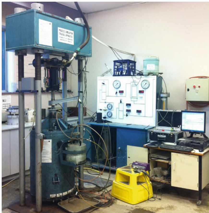
Fig. 7 Large-scale triaxial test facility at UOW
