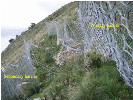
Fig. 6 Only one block over passed the primary barrier and impacted on the secondary one
