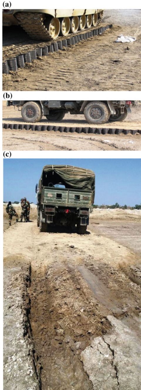
Fig. 16 a Unpaved geocell reinforced path with tracked 50T vehicle after several passes, b unpaved geocell reinforced track with wheeled loaded vehicle after several passes, c comparison between the unreinforced, unpaved track and reinforced, unpaved track
