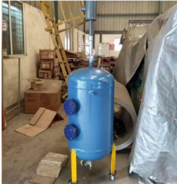
Fig. 6 Cylindrical pressure vessel with color-coded paint
