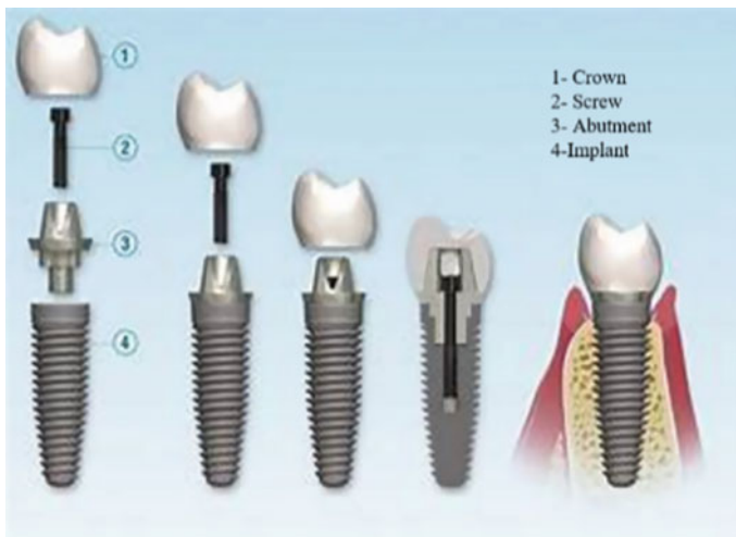
Fig. 8 Different parts of tooth abutment implant. Source [24]
