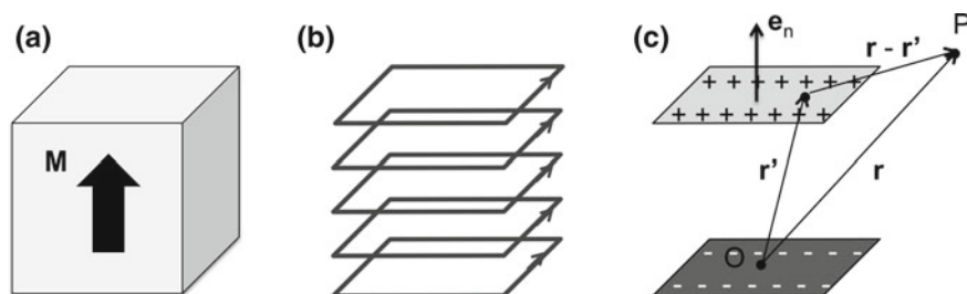
Fig. 7.13 Equivalent approaches for the calculation of the magnetic stray field emanating from a uniformly magnetized magnet with a square section a fields produced by an equivalent distribution of currents b and an equivalent distribution of charges c
