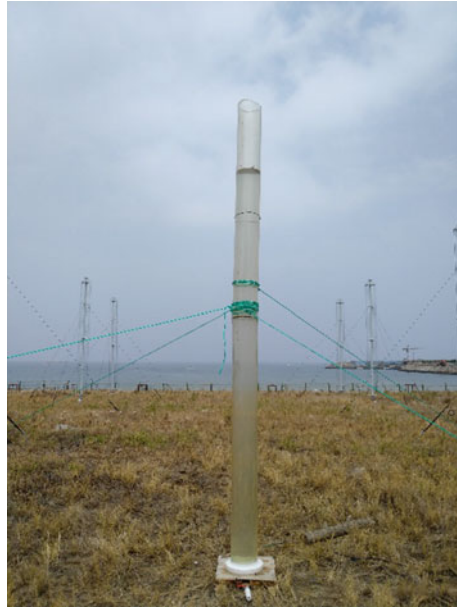
Fig. 7. Photograph of the fabricated seawater antenna
