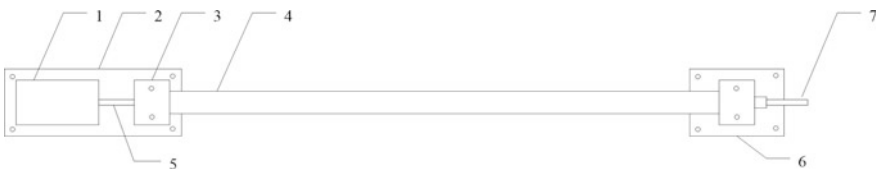
Fig. 2. Structural of the new hull structure long base stress sensor
