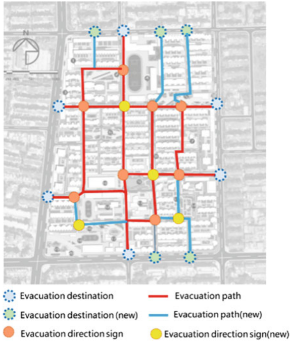
Fig. 6. Sketch of evacuation path after optimization
