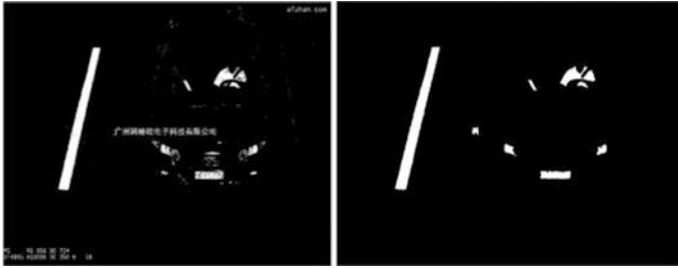
Fig. 9. Images before and after morphological processing
