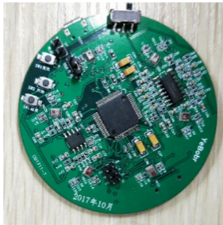
Fig. 4. Circuit board diagram of the microphone array
