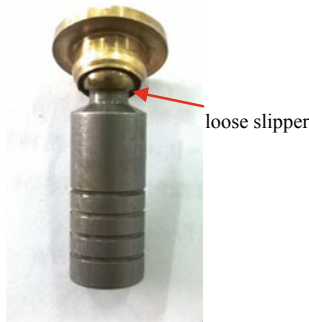
Fig. 1. Fault of loose slipper
