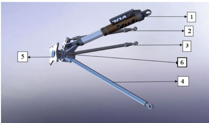
Fig. 2 CAD model of the multilink independent rear suspension system. (1) Air Shox (2) Upper control arm (3) Lower control arm (4) Trailing arm (5) Wheel Hub (6) Knuckle
