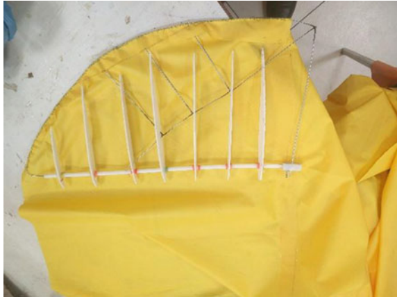
Fig. 4 Wing with wire mesh and slices of styrofoam sheets cut in the desired airfoil shape
