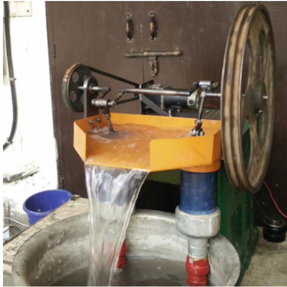
Fig. 4 Assembled solar-powered treadle pump
