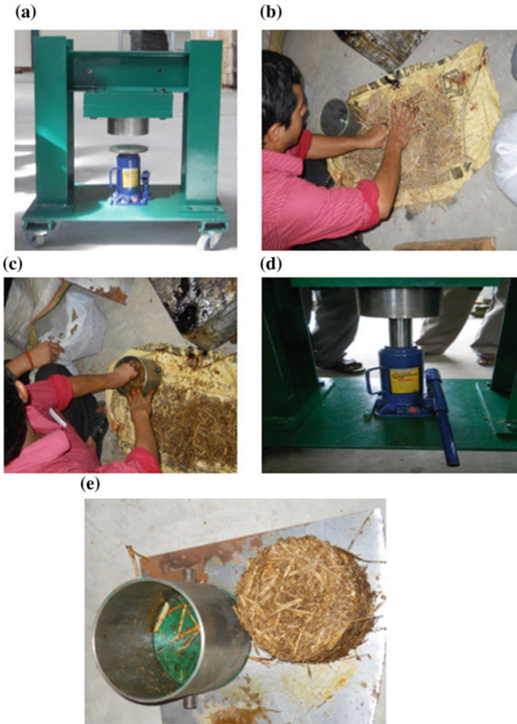
Fig. 3 Operational model of feed block making machine developed by RuTAG; a Feed block production machine; b Preparation of mixture for feed block; c filling the cylinder manually; d Hydraulic jack; e Feed block
