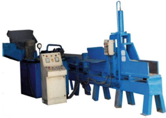
Fig. 1 Feed block making machine provided by Indian Agriculture Research Institute (IARI) [46]
