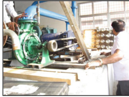
(b) Testing of the pump for Power generation at Laboratory
