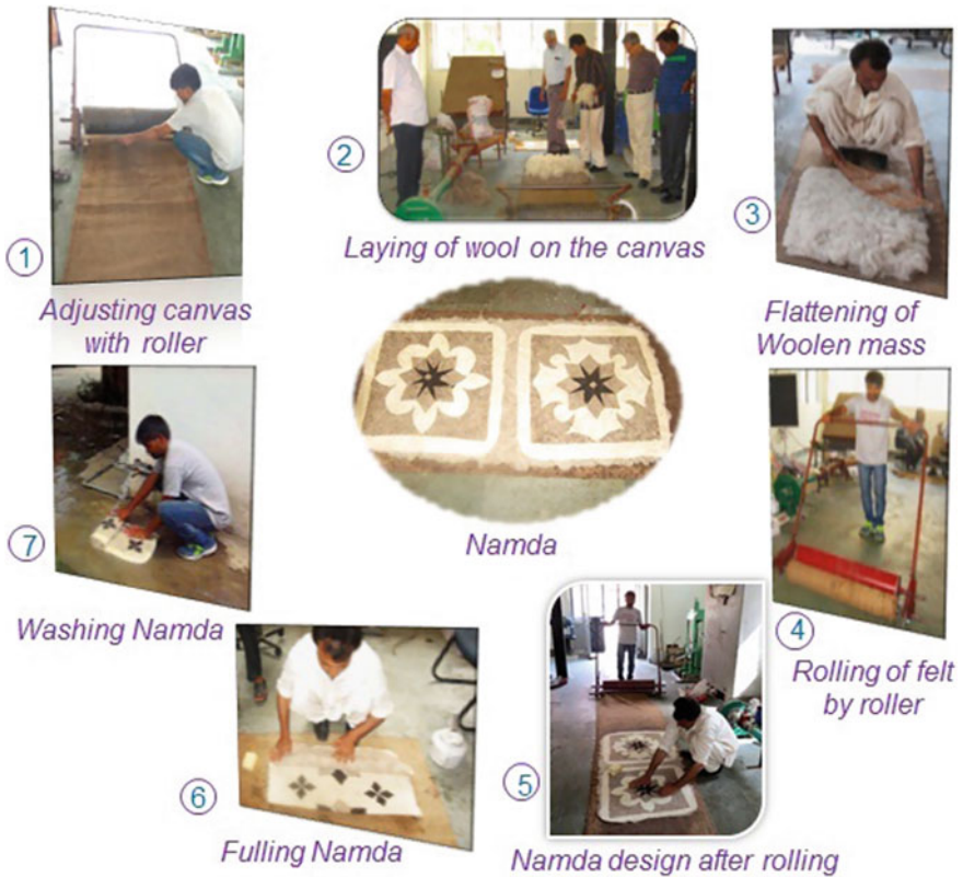
Fig. 7 Complete processing for making felt using mechanized rolling devices [6, 7]
