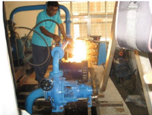
(c) Testing of the pump for Power generation at Laboratory
