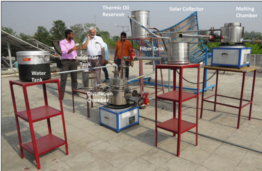
Fig. 12 Experimental setup of solar energy based turpentine oil extraction unit [14]
