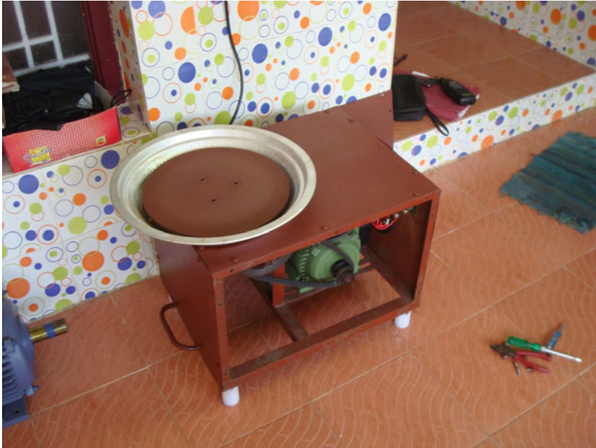
Fig. 7 Automatic potter's wheel developed by RuTAG
