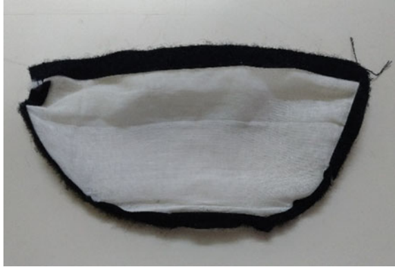
Fig. 2 Velcro stitched around a strip of nanofilter
