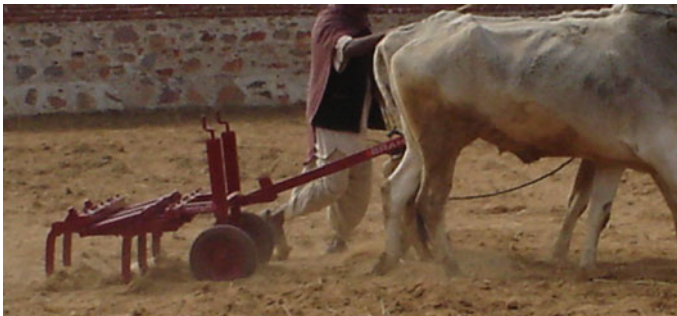
Fig. 10 Existing bullock driven tractor ('Brahmpuri' Model)
