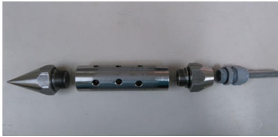
Fig. 9 Split view of the probe
