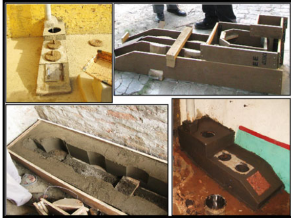
Fig. 2 Manufacturing of the stove using mould
