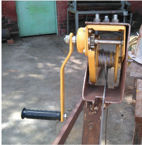
Fig. 10 Winch-wire rope device
