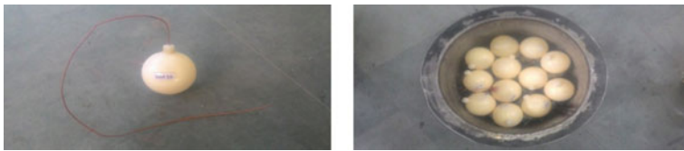
Fig. 1 Photograph of EPCM and arrangement in TES tank
