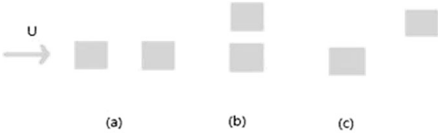
Fig. 1 Two square cylinders in cross-flow: a tandem configuration; b side-by-side configuration; and c staggered configuration
