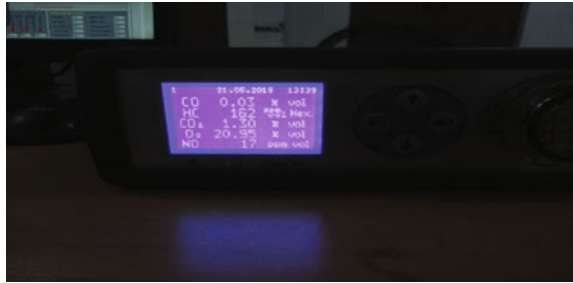
Fig. 5 Calibrated values in gas analyzer
