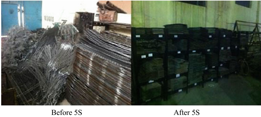
Fig. 3 Raw material was placed on floor, after 5S it was placed on racks with naming [12]
