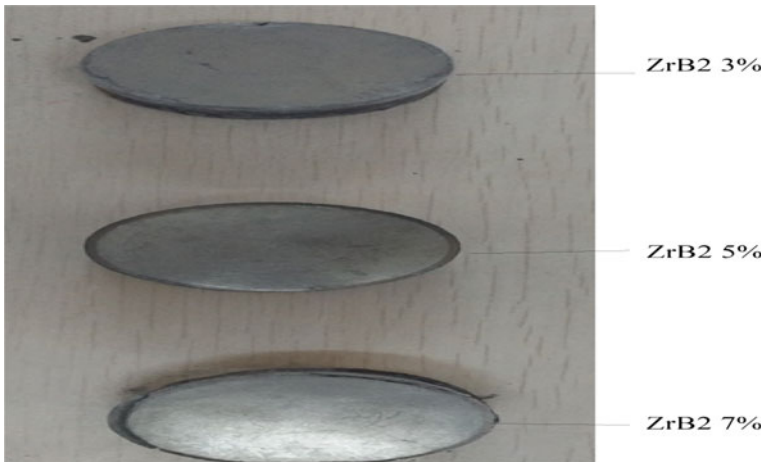
Fig. 3 Different composition of \text{Al}_2\text{O}_3 and \text{ZrB}_2 in Al
