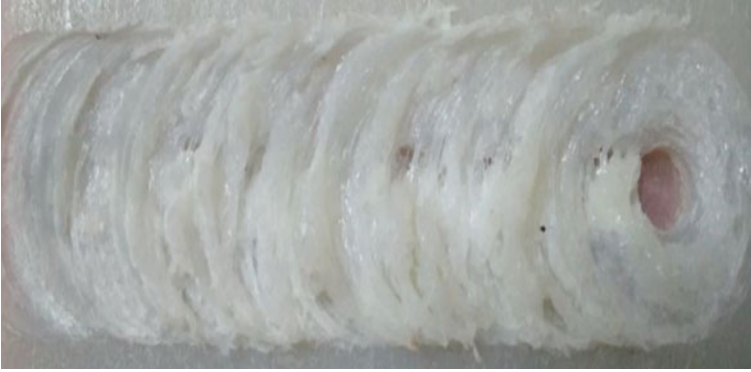
Fig. 5 Typical macrograph of weld crown at tool traverse speed of 0.6 mm/s, tool rotational speed of 600 rpm, and tilt angle of 2°
