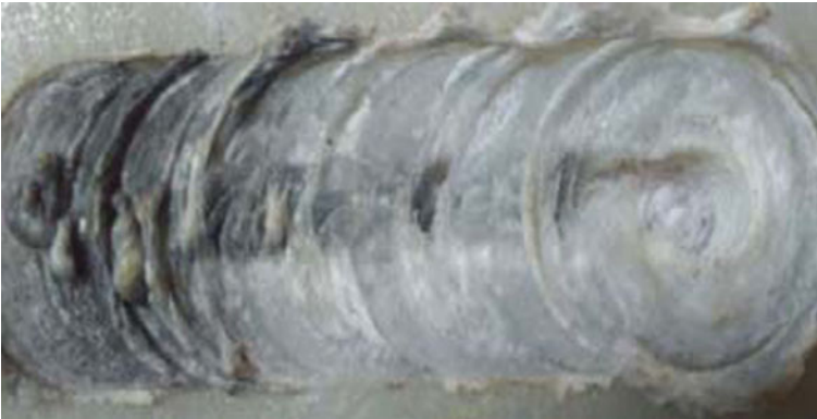
Fig. 6 Typical macrograph of weld crown at tool rotational speed of 1000 rpm, tool traverse speed 0.2 mm/s, and tilt angle of 2°
