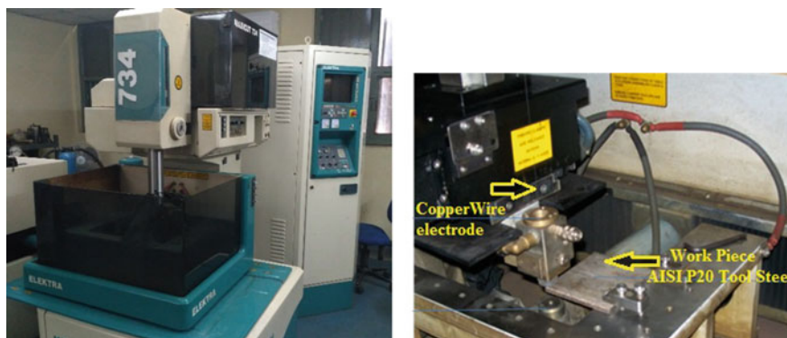
Fig. 1 Wire electric discharge machining with tool and workpiece
