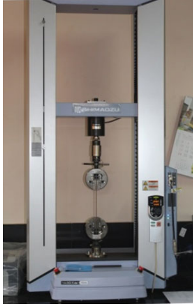
Fig. 1 Tensile testing according to ASTM D3039
