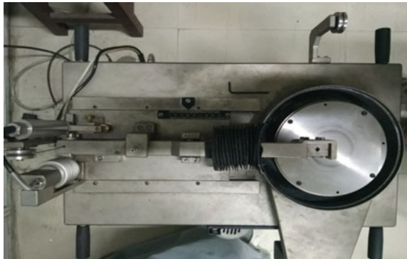
Fig. 2 Wear testing set-up (pin-on-disc)
