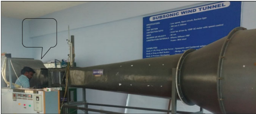
Fig. 6 Wind tunnel setup to test at subsonic speed
