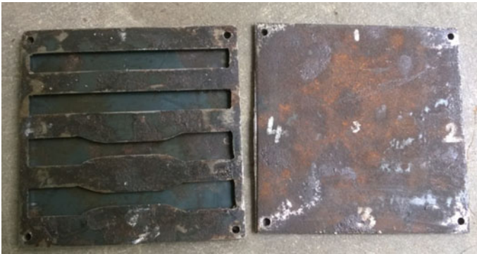
Fig. 9 Die for the preparation of the composite
