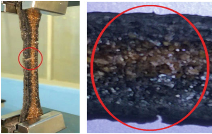
Fig. 13 Tensile testing on the composite
