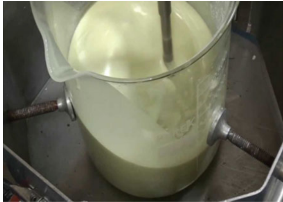
Fig. 3 Mechanical stirring (epoxy + ZnO particle)
