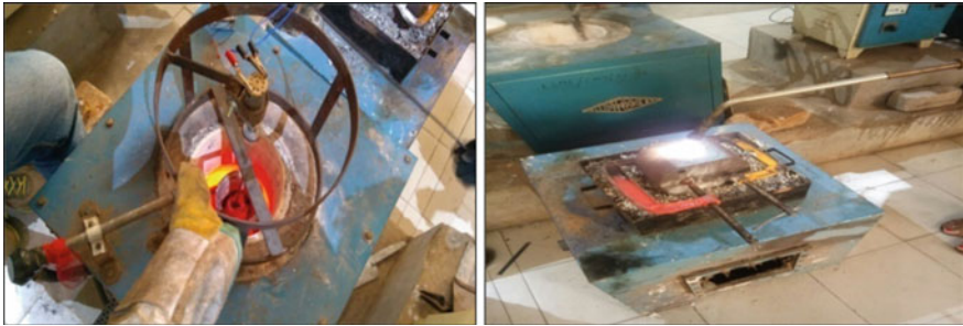
Fig. 1 Schematic view of the furnace along with stirrer and preheating setup of the die
