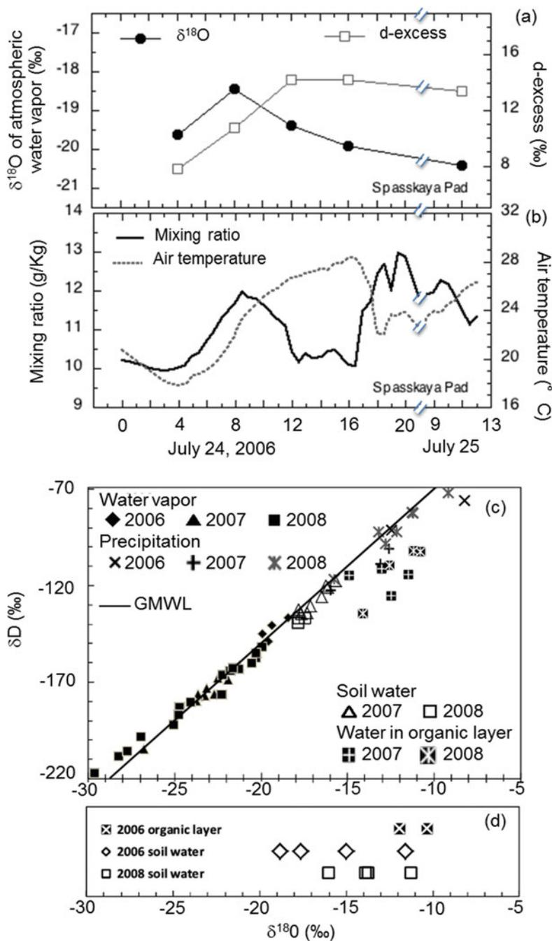
**Fig. 6.7** Typical diurnal variations of  $\delta^{18}\text{O}$  and d-excess (a) of atmospheric water vapor and air temperature and mixing ratio at 24 m (b) observed at Spasskaya Pad on fine day and  $\delta\text{D}$ - $\delta^{18}\text{O}$  plots for various water samples (c) and  $\delta^{18}\text{O}$  of surface soil water (d). (Reproduced from Ueta et al. 2013)
