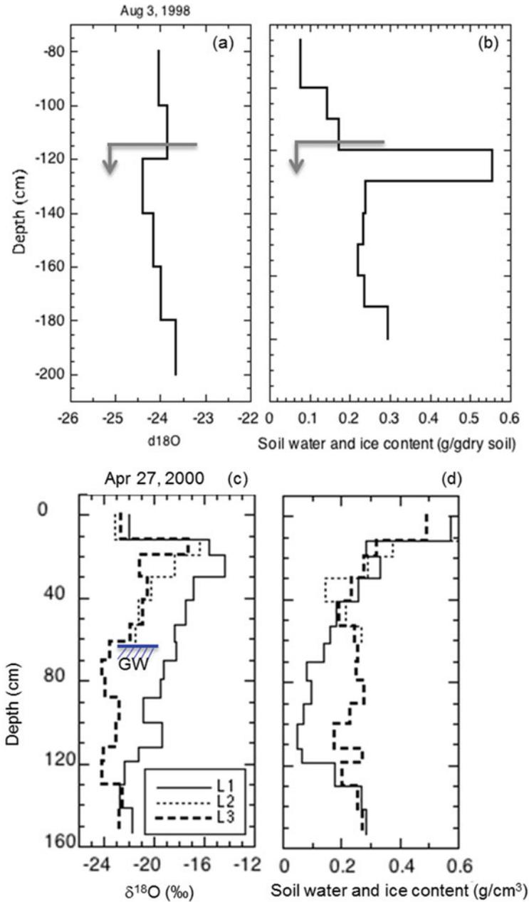
**Fig. 6.3** The  $\delta^{18}\text{O}$  value (a) and water content (b) of soil moisture (water and ice) in the layer from 80 to 200 cm observed on August 3 in 1998 and those from surface to 150 cm observed on April 27 in 2000 (c and d). Soil layer shown in (a) corresponds to lower half of active layer (80–140 cm) and upper part of permafrost (140–200 cm). GW in (c) is a water table of talik which was formed after heavy rainfall in 1999. (Data were modified from Sugimoto et al. 2003)
