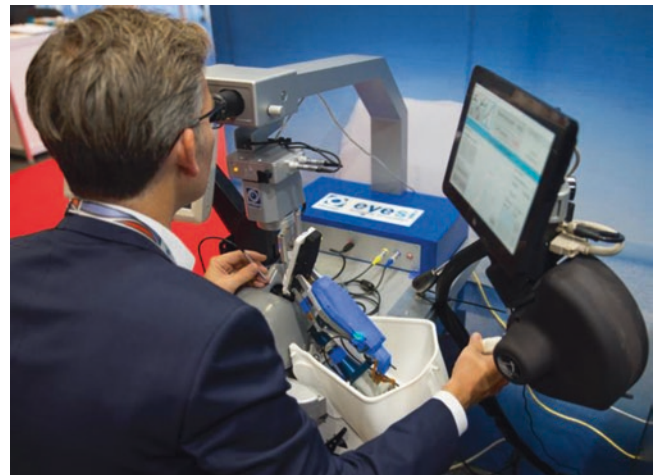
Fig. 11.7 Robotic eye surgery training using the Preceyes Surgical System linked to the virtual reality simulator, Eyesi Surgical (VRmagic GmbH, Mannheim, Germany)
