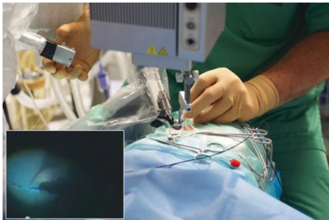
Fig. 11.6 Robot-assisted cannulation of a retinal vein in the pig eye. The surgeon can be seen holding the robotic motion controller in the right hand, which controls the robotic instrument manipulator, and an endoillumination light pipe in the left hand. Inset: cannulation of a retinal vein and injection of thrombolytic agent
