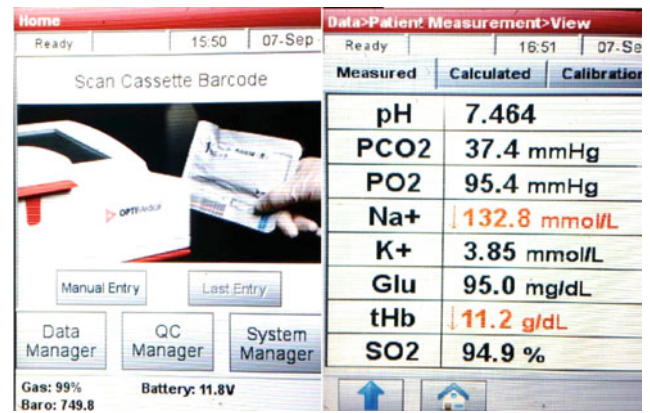
Fig. 6 The main menu of the blood gas analyzer (left) and a patient result (right)
