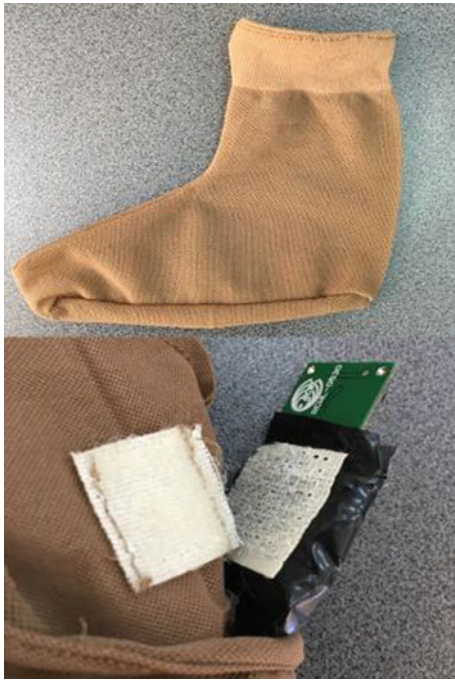
Fig. 2 Textile material and fastening system
