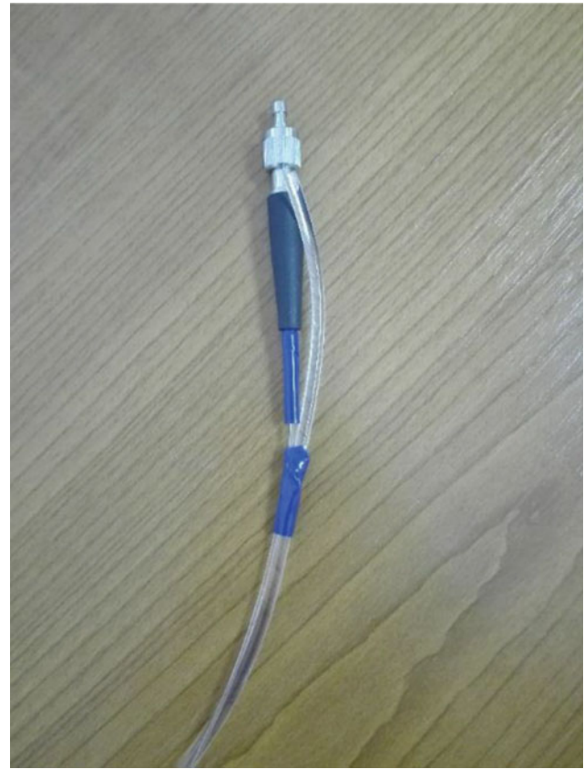
Fig. 7 Photograph of the side-polished fiber optic salivary sensor, based on filtering the incident light coming from a side-emitting fiber
