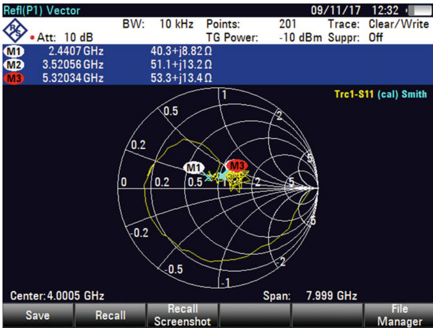
Fig. 9 Measured impedance of proposed antenna
