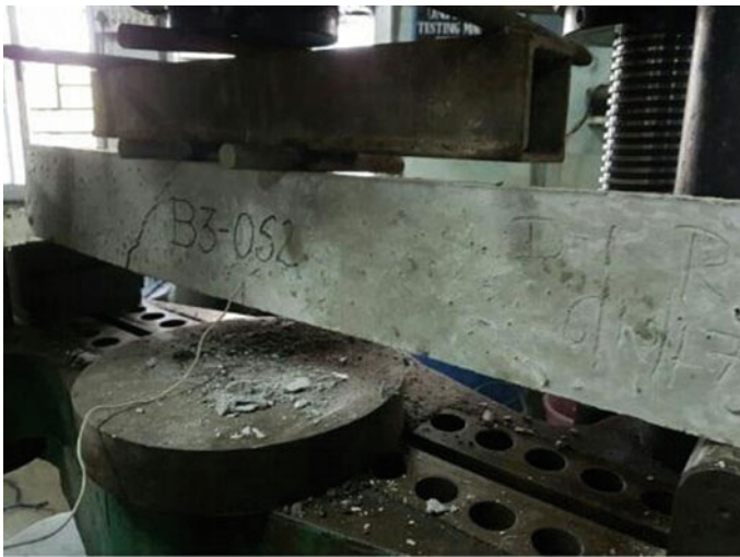
Fig. 11 Damaged beam 3 (OS 2) with visible cracks
