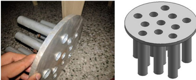
Fig. 3 Top plate, salt cylinder assembly and 3D model of full assembly of oil-based tank
