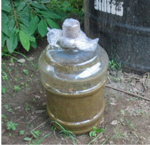
Fig. 2 Batch feed Digester
