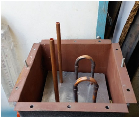
Fig. 6 MTC placed in the outer casing
