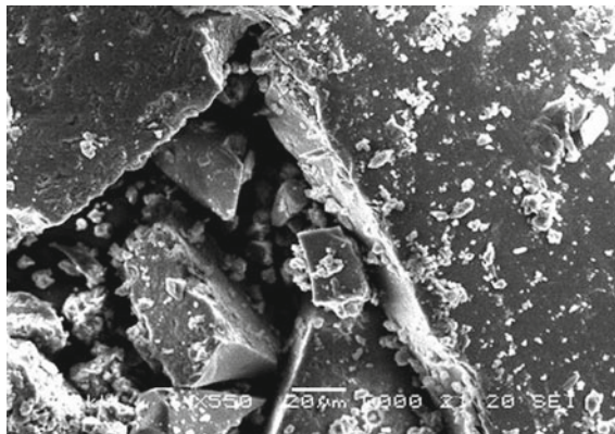
Fig. 4 SEM image of CuO nanoparticles [3]
