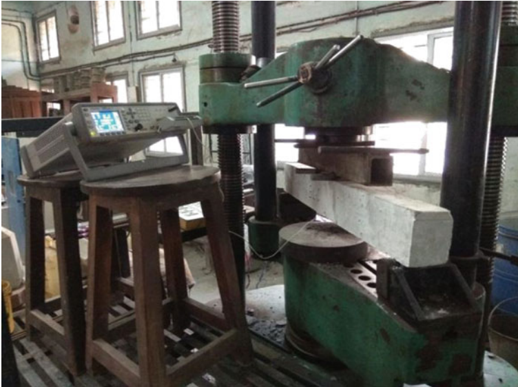
Fig. 4 Beam 1 (control) loaded on UTM and connected to LCR meter
