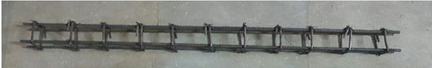
Fig. 2 Reinforcement of control beam
