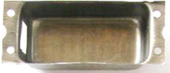
Fig. 1 Part drawing of rectangular deep draw part
