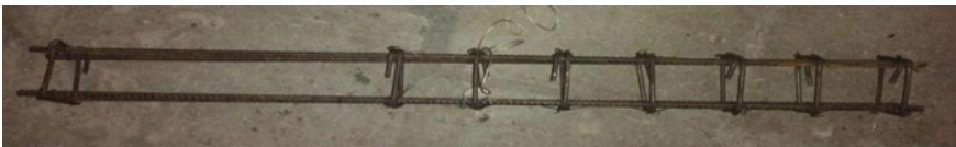
Fig. 3 Reinforcement of shear deficient beams
