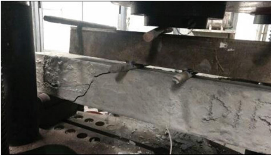
Fig. 9 Damaged beam 2 (OS 1) with visible cracks
