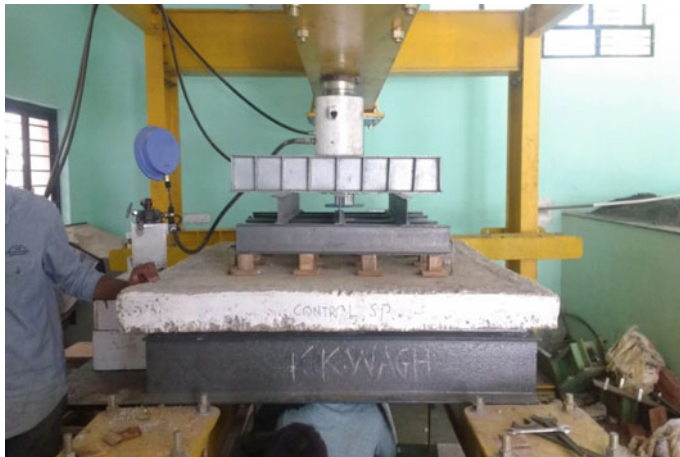
Fig. 7 Flexural test setup
