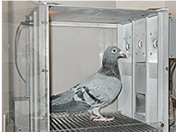
Fig. 3 An operant chamber for pigeons. During an experiment, pigeons are placed in the operant chamber. A plastic disk, generally referred to as a “key”, is located in the upper part of the front panel. Pigeons are trained to peck the key that can be illuminated with different colored lights. Reinforcers are delivered through a grain feeder which is shown in the lower part of the front panel. Pigeons can earn access to a food hopper filled with grains (i.e., the reinforcer) for a few seconds for pecking the illuminated keys
