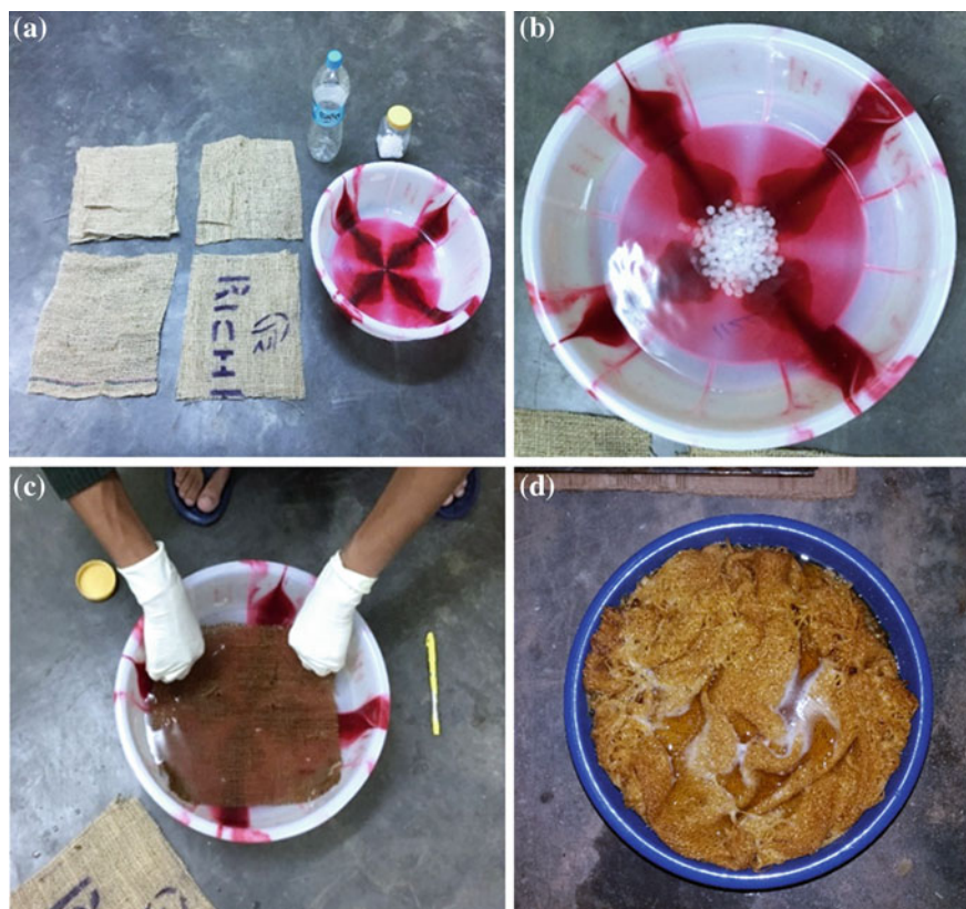
Fig. 2 Chemical treatment of natural fiber a preparation of solution, b NaOH solution, c alkaline treatment of fiber with NaOH, and d alkaline treatment of fiber with NaOH, KOH, and H 2 O 2
