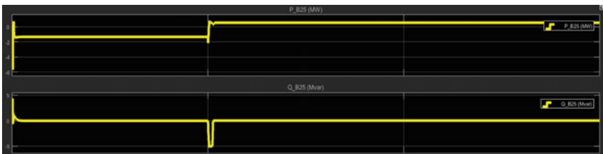
Fig. 7 Graph showing real and reactive power at 25 kV bus before-fault, at-fault, and after-fault
