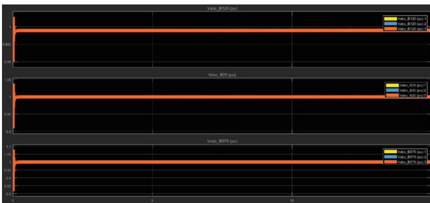
Fig. 2 Graph of output voltages at various buses to change in wind speed
