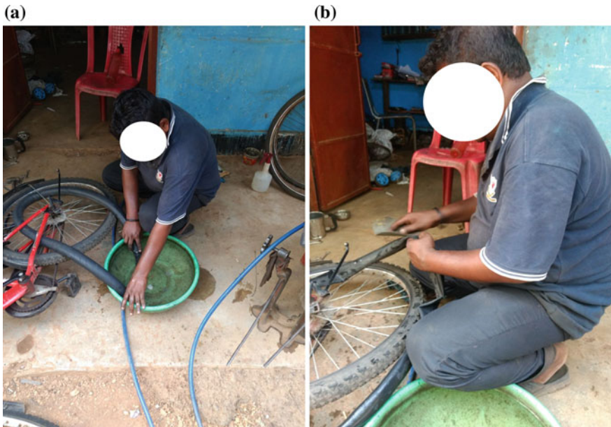
Fig. 43.1 A bicycle repairer a locating puncture and b repairing puncture
