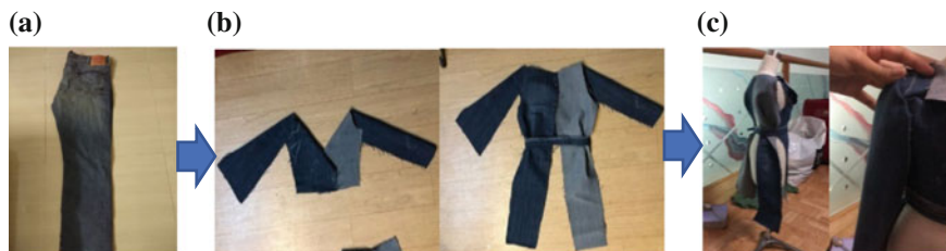
Fig. 19.1 a Original garment, b opening the seams and placement of panels, c draping on a standard women's dress form
