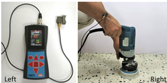
Fig. 47.2 Hand-arm vibration meter connected with the triaxial accelerometer (left image) and triaxial accelerometer on the wrist of the operator during use of polishing machine (right image)
