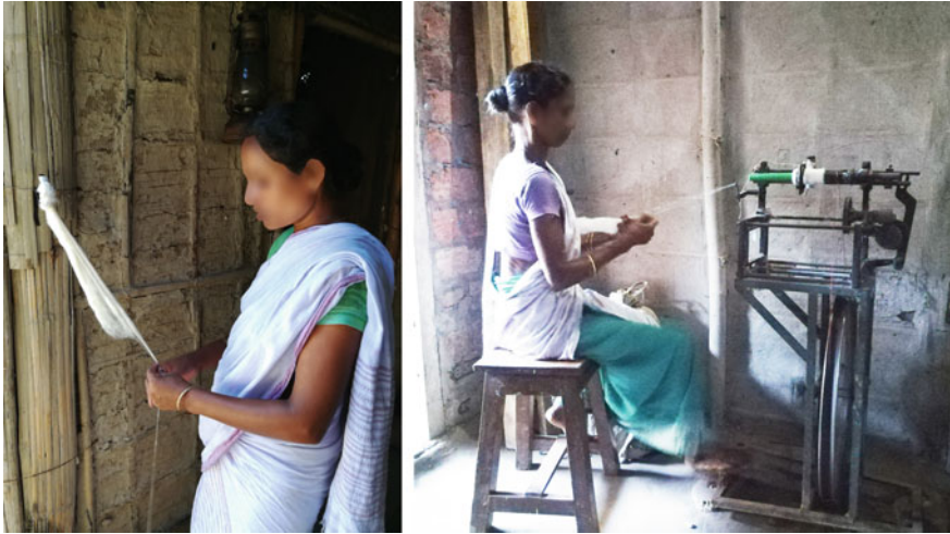
Fig. 70.3 Hand spinning process and semi mechanized spinning process
