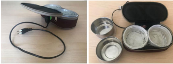
Fig. 84.4 A student project, for heating cold lunch food in an easy and cheap way, involving electric circuits and components, done by mechanical students
