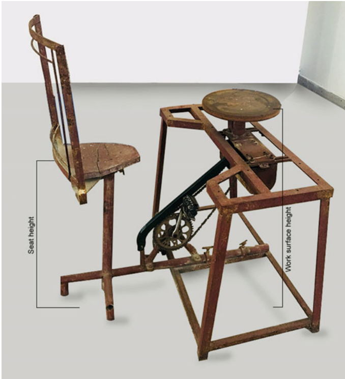
Fig. 35.1 Pottery wheel designed by IIT Kharagpur
