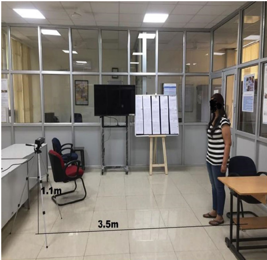
Fig. 49.1 Placement of kinect sensor w.r.t. chair position
