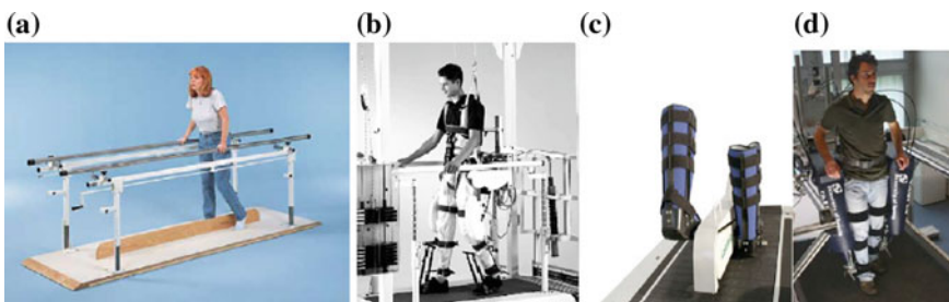
Fig. 39.2 a Parallel bars, robotic mobility training devices: b Lokomat, c LokoHelp and d Lopes. Source Martins et. al
