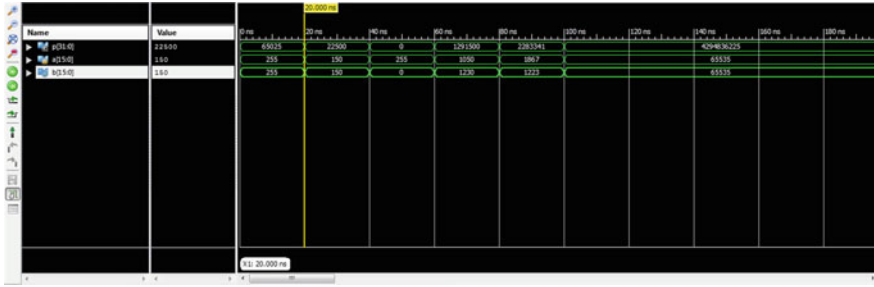
Fig. 6 Simulation results of 16-bit modified array multiplier
