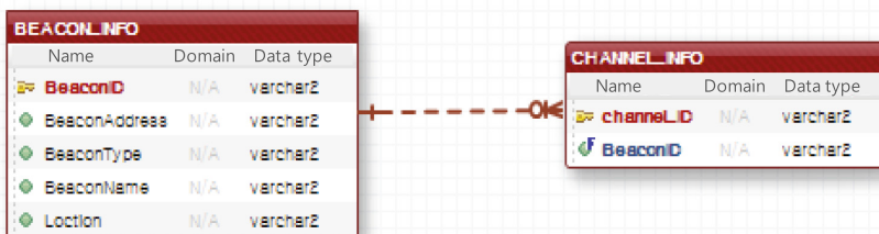
Fig. 5. Beacon and channel database table
