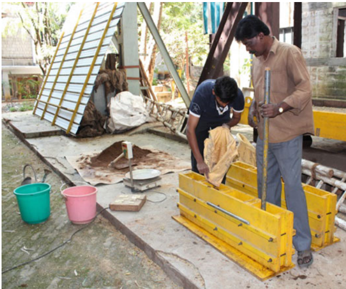
Fig. 6.3 Casting of rammed earth shear test specimen
