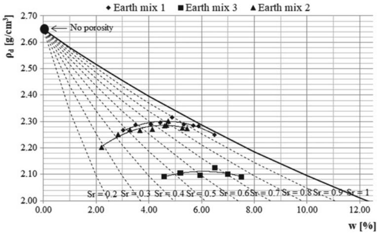
**Fig. 17.4** Compaction curves for the static pressure of 100 MPa
